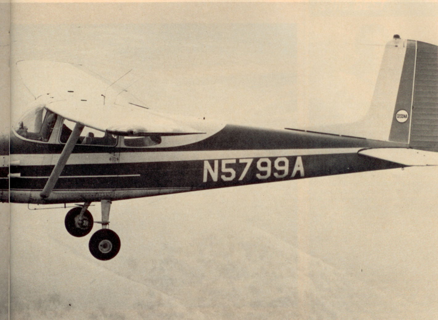
Unswept tail, lack of rear window identify "original" Cessna 172, first produced in 1955 and still popular on the used, four-seater market.
